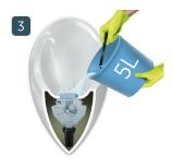
Flush (fast pour) with 5 litres of warm water to ensure waste trap clears.
